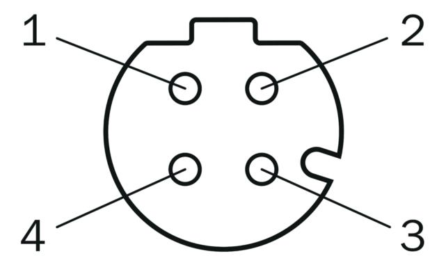
M12 female connector, 4-pin, D-coded
