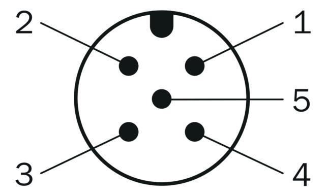
Connector M12, 5-pin, A-coded
