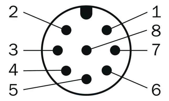
Connector M12, 8-pin, A-coded
