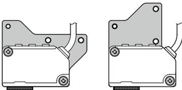
Two M4 (length 28 mm 1.102 in) screws with washers are attached.
