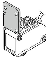
Two M4 (length 30 mm 1.181 in) screws with washers are attached.
